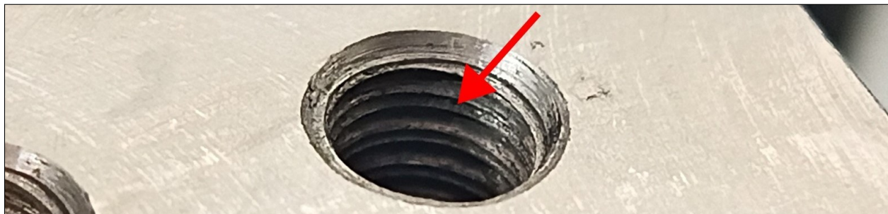
Figure 6: Double thread appearance from cold form taps. This crest recess decreases with higher percent engagement.
