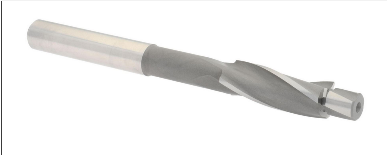
Figure 8: Pilot counterbore commonly used for creating the counterbore for socket head cap screws.
