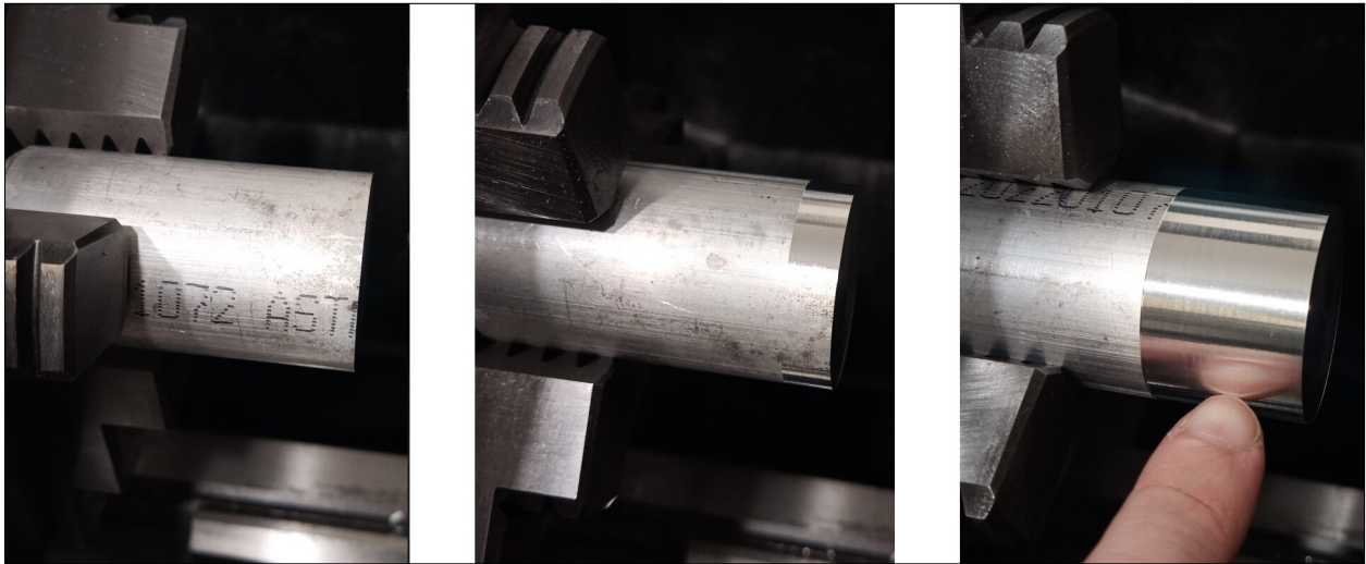
Figure 2: A 1.5 in aluminum bar is turned by taking .005 in off the diameter. Notice this doesn't quite clean up the surface (center image). This bar required taking .012 in off the surface to leave a nice finish. If a nice surface finish is preferred at 1.5 in , the next larger stock size is required and results in higher material costs and more machining time.
