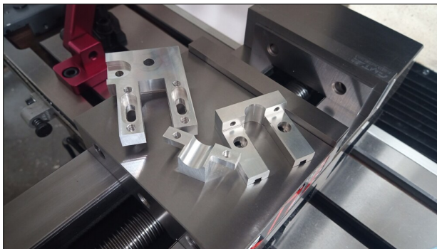
Figure 13: Complex parts requiring different machining operations.
